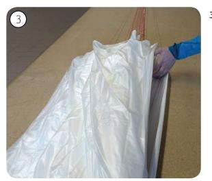
**4.** Pull the base from one line attachment point to the next along the seam to the side you are sorting and smooth the crossed panel. A line separator and a weight will help to secure
