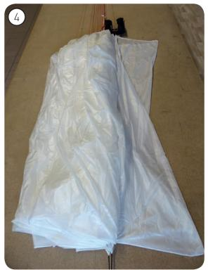
7. The SALSA is a cruciform rescue parachute with four corner points, so lay out the canopy with one corner at the bottom, one on the left, one on the right and one on top.
