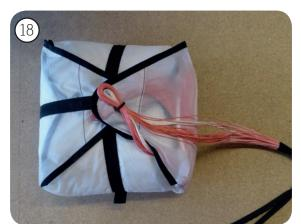
16. Starting at the main riser, loop the line bundles in the shape of a figure-eight. Use silicone-based rubber rings to fix the line bundles.
