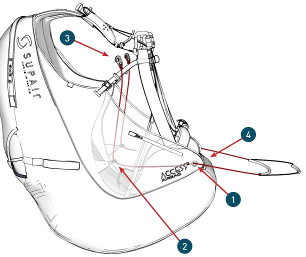
Simulate the speed-bar/accelerator's functionality by sliding the cord back and forth.
