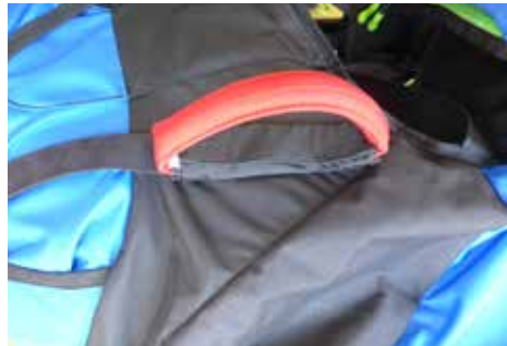
Position the handle in its folding sleeve. It may not protrude from the harness.
