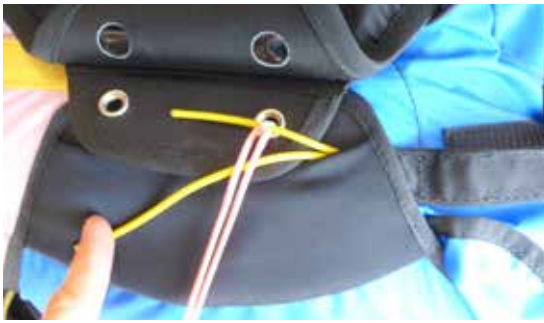
Push the yellow cable through the loop and gently pull the cord out.
